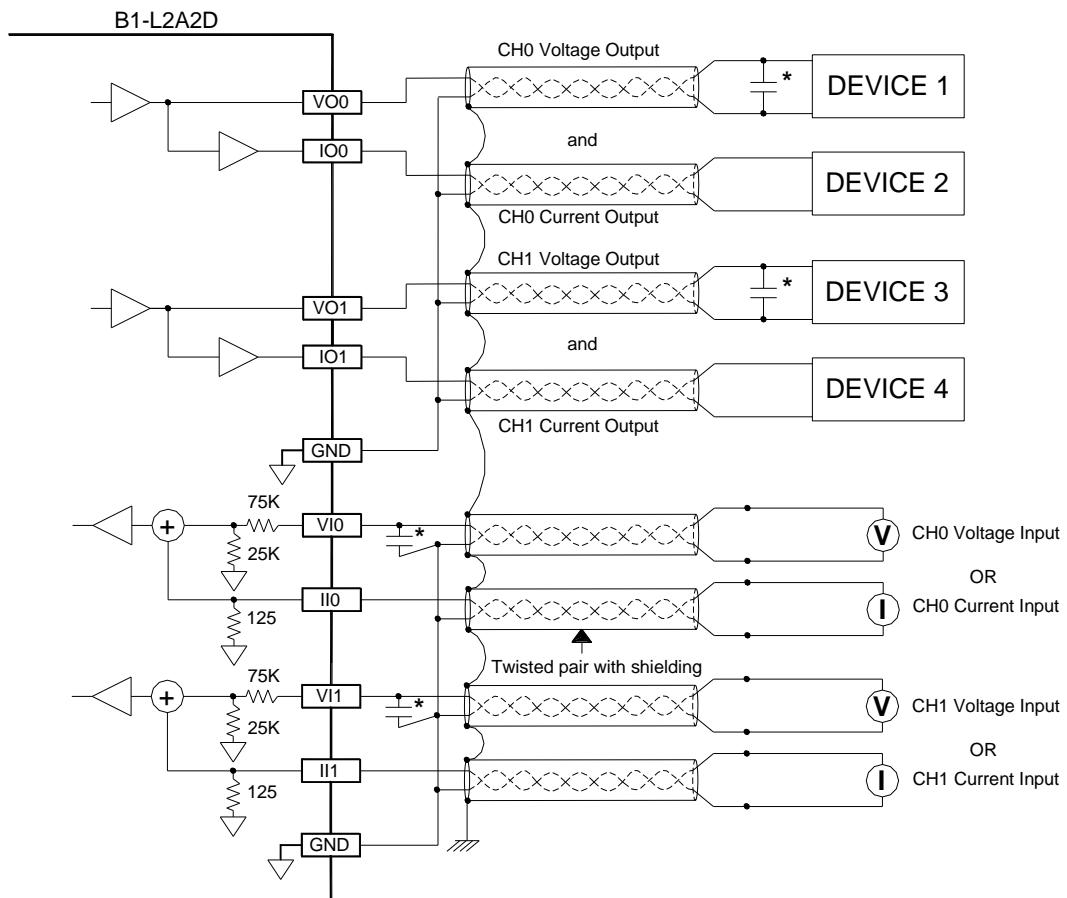
\*0.1~0.47uF capacitor (to filter noise) ..... Advice to install, but not necessary!!
