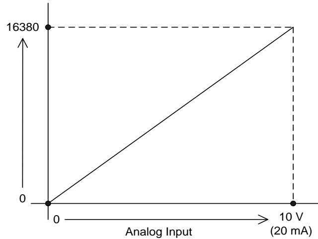
Figure 2 : Analog Output Characteristics Curve
