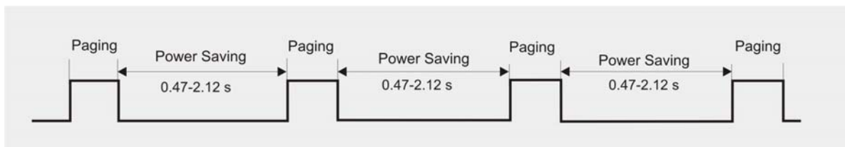
Figure 9: Power saving and paging in GSM networks
